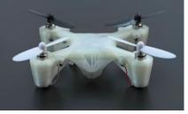
Quadcopter the 3D-printed Quadcopter communicates with an existing embedded pcb; magnetic connections provide contact between the pcb and the printed silver interconnections
